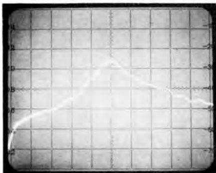
Typical frequency response measured on an Anritsu MS62D spectrum analyser. Vert - 10dB/div. Hor. 100MHz/div. C/F 1296MHz. Gain 14dB.
